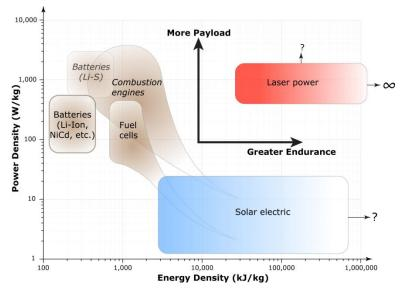
LaserMotive has demonstrated wireless power systems with a receiver specific power as high as 800 W/kg. By comparison, lithium-ion batteries used in small UAVs are generally used with a specific power in the range of 200-500 W/kg.
