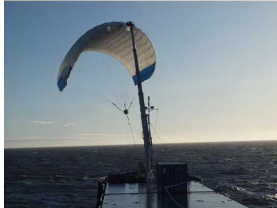
Fig. 32.7 The system is ready for take-off when the kite is fully inflated, checked and the mast is in take-off position. A challenge is the kite check after inflation. An automated check for lines and canopy is difficult to develop. A possible solution is a camera which can be used by a human operator. Then a control center does not necessarily have to be at the same location as the AWES
