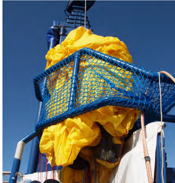
Fig. 32.6 A cone (tubing and textile mesh) close above the stowing hatch helps to further compress the kite volume. Below the cone the reefed kite has the right dimension to slide into the stowing compartment. When the hatch is closed the airborne system is inside the robust shelter and therefore safe. The components outside the shelter withstand all ambient conditions
